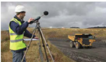
Acoustic monitoring of 777F dump trucks
